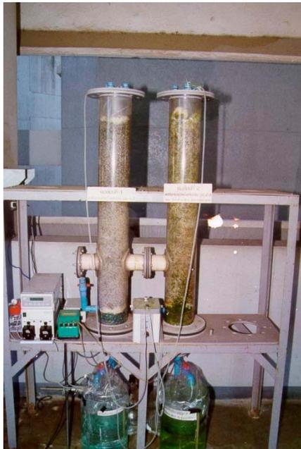
Bioleaching of copper from low-grade copper sulphide ores by *Thiobacillus ferrooxidans* in a column leaching
