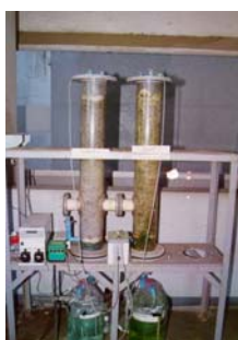
Bioleaching of copper from low-grade copper sulphide ores by Thiobacillus ferrooxidans in a column leaching
